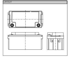
This battery type must never be installed suspended by their handles
